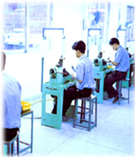
投影機檢驗 PROFILE PROJECTOR MEASURING
